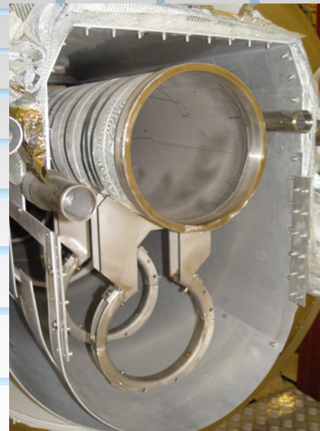
Quadrupole support structure (shown without the quad)
