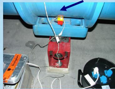
Measurements on the stability of the jacks were performed on 4 modules in total: 2 stand-alone cryo-dipoles (for reproducibility checks), one connected to the other modules in the ring and one low beta cryo-dipole (ALICE interaction point).
