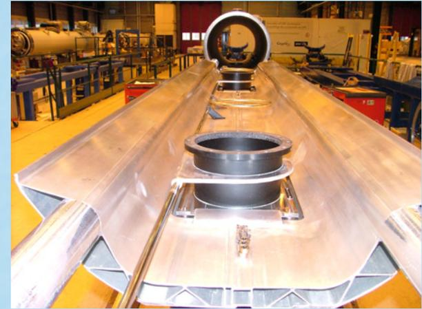
LHC standard cryo-dipole installed in the 3-4 arc section. Note the small concrete interface between the jack and the tunnel floor as compared with low beta quads (next slide).
