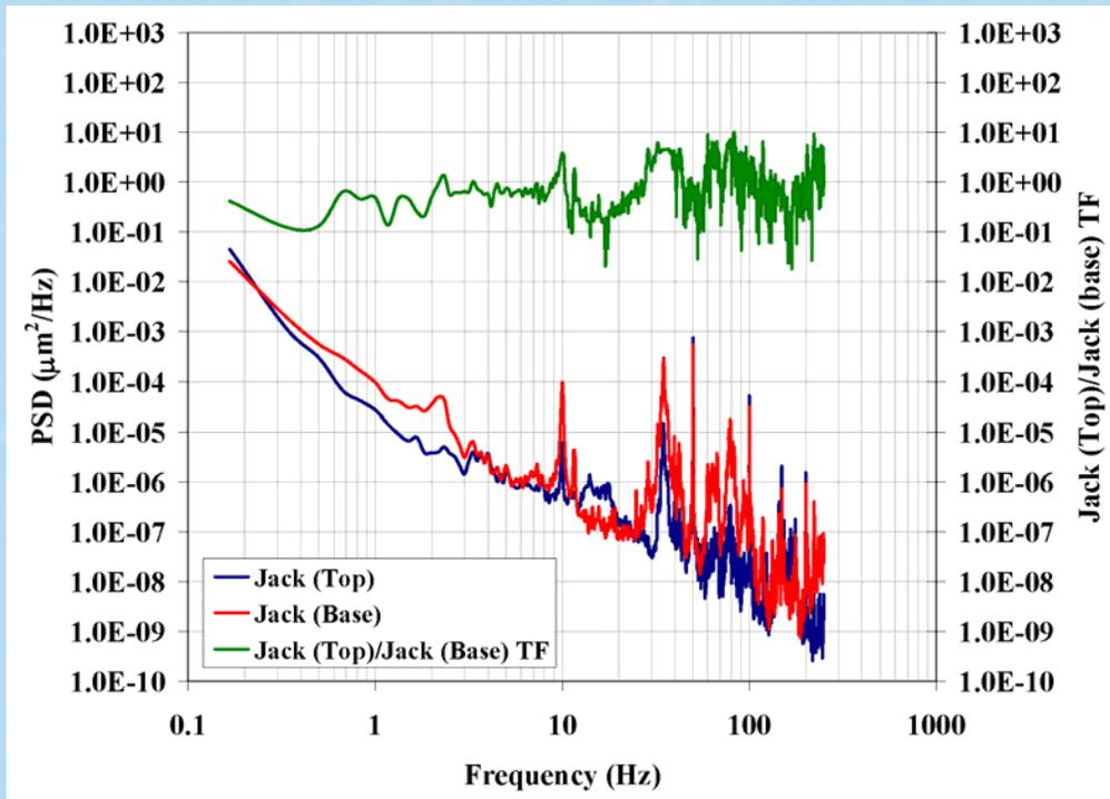
**Conclusion:** For the ILC supports, one should concentrate on the optimization of the interface between the tunnel floor and the jacks.
