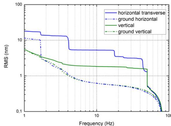
**Vertical is more stable than horizontal transverse, however LHC tunnel is a very quiet site, in the order of only a few nm rms @  $f > 1$  Hz.**
