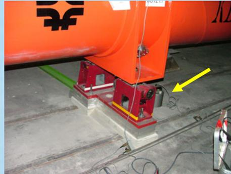
Standard FFT techniques were used to deduce power spectrum density (psd) and integrated spectra resulted in the displacement (in nm) at  $f > 1$  Hz. For more information, please click on:
