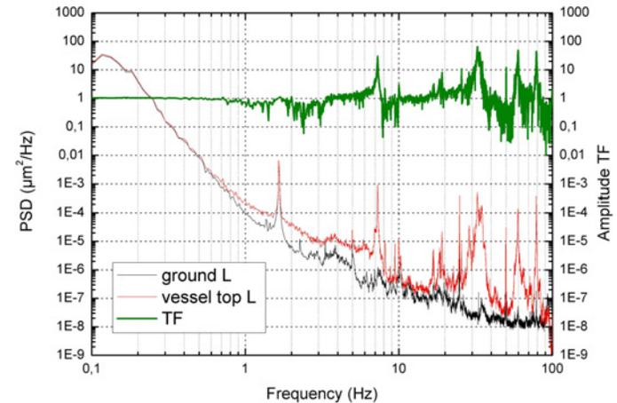
Comparison of ground spectra vs. vessel top in horizontal transverse, longitudinal and vertical directions clockwise (seismometer measurements) for the low beta modules.
