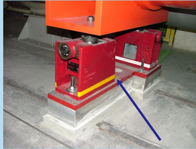
View of the alignment jacks. Note the enlarged contact plate between the jacks and the concrete slab for better surface contact, and hence stability.
