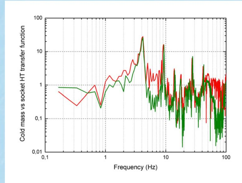
Cold mass transfer function (horizontal transverse) comparison
