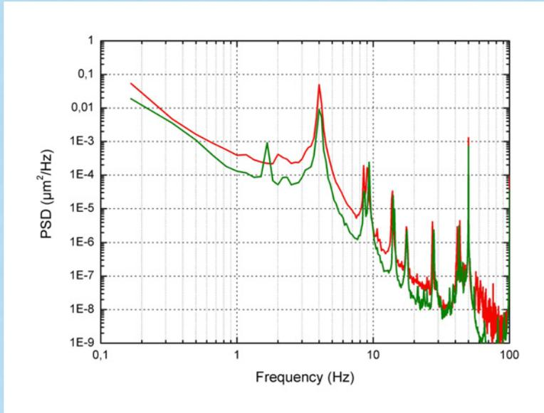
Cold mass spectra (horizontal transverse) of two dipoles
