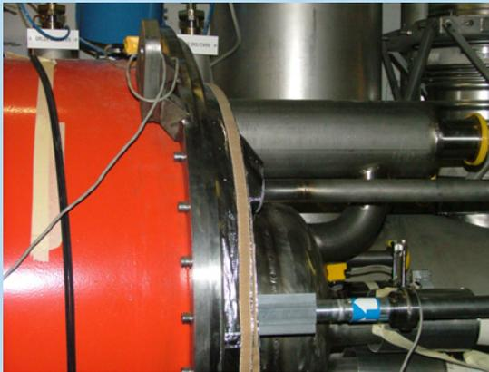
the cold mass motion is dominated by the large amplitude module rocking modes. In dipoles seems not very well supported internally: two modes at 8 and 14 Hz are visible in the cold mass PSD only. In the case of the low beta quadrupole, the lowest modes are seen at 16 and 18 Hz.
