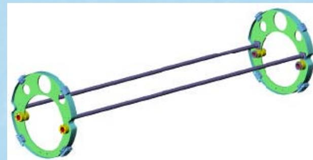
Composite spider-like cold mass support, designed for better support .
