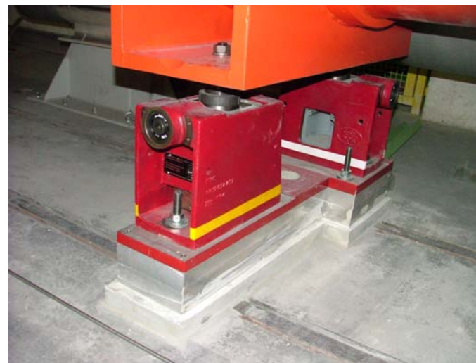
View of the alignment jacks. Note the enlarged contact section and the extra layer of concrete.
