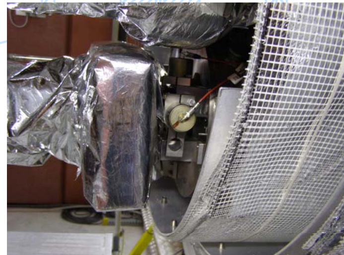
Geophones installed on the quad front face
