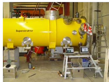
Fig.2: TESLA type II cryomodule setup in Hall 3 in DESY for vessel vs. ground measurement.
