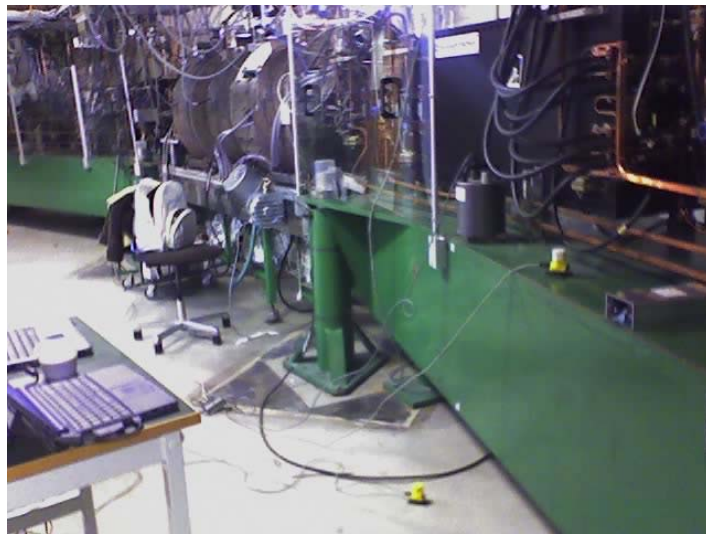
Figure 1: Partial view of a MAXLab girder. A Güralp CMG-6TD seismometer was placed on the girder for the vibration measurements. Simultaneously, two vertical and horizontal geophones repeated this measurement for a snapshot period of few minutes.
