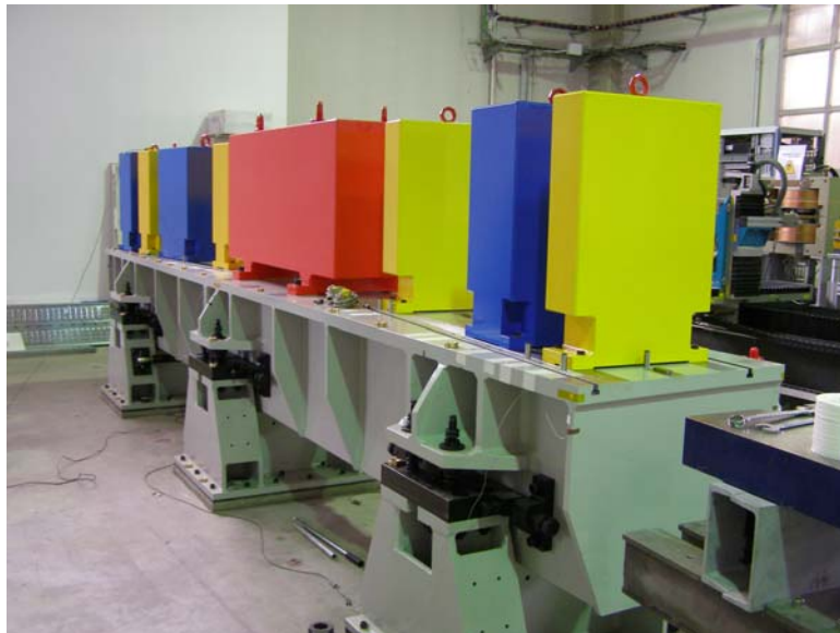
Figure 1: Magnet girder prototype of ALBA, fully attached to the floor and the magnet dummies. The red structure in the center is a dipole (dummy), the blue are quadrupoles and the yellows are sextupoles.
