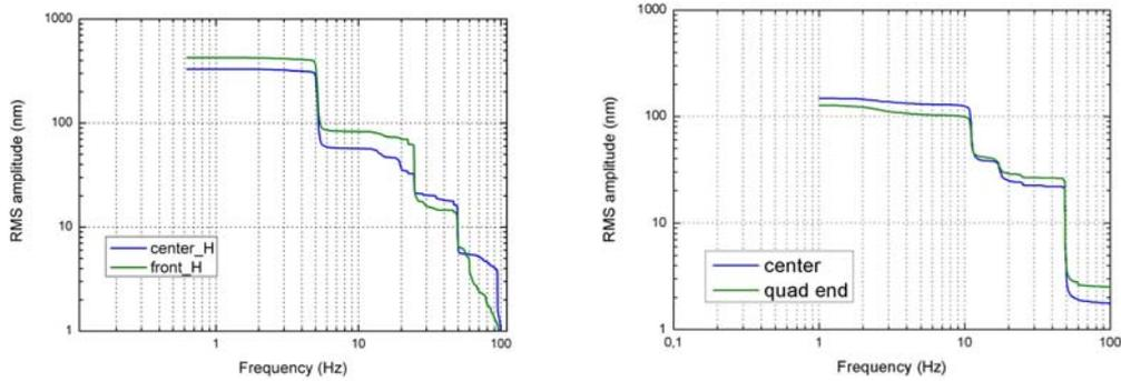
**Figure 3:** Quadrupole end vs. center horizontal rms comparison: inside the HeGRP with the module sitting on concrete blocks (left). On top of the vessel with Module 6 installed on the CMTB (right); in this configuration, a slightly larger amplitude was measured at the center.
